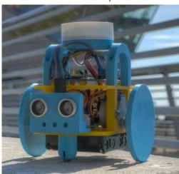
Creating physical devices is a great way to learn. The **Hull Pixelbot** grew out of a recognition of this, aiming to provide a platform that is simple to use, easy to extend and, above all, cheap to engage with. The hardware required to create the base platform can be purchased for around ten pounds.
