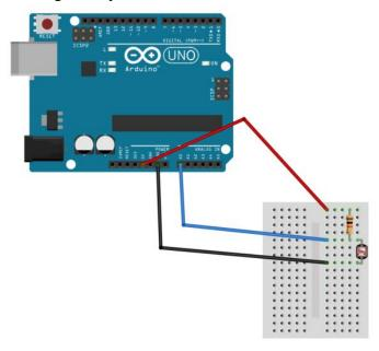
This is the potential divider circuit implemented on breadboard.
