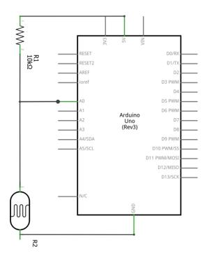
If that sounds hard to understand, consider what happens in the dark. In the dark the photocell has a resistance of 10,000 ohms (the same as the resistor). This means that half the voltage will be across the photocell and the other half will be across the resistor. This means that the A0 input should be at around 2.5 volts.
