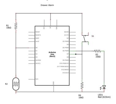
This is the circuit of the complete alarm. The button (S1) is connected to pin D7, which is configured as an input. The LED (LED1) is connected to pin D6 which is configured as an output.
