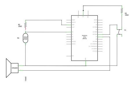
This is the circuit diagram that should do all this. The light sensor is connected to A0, the sounder is connected to D7 and the button is connected to D6.
