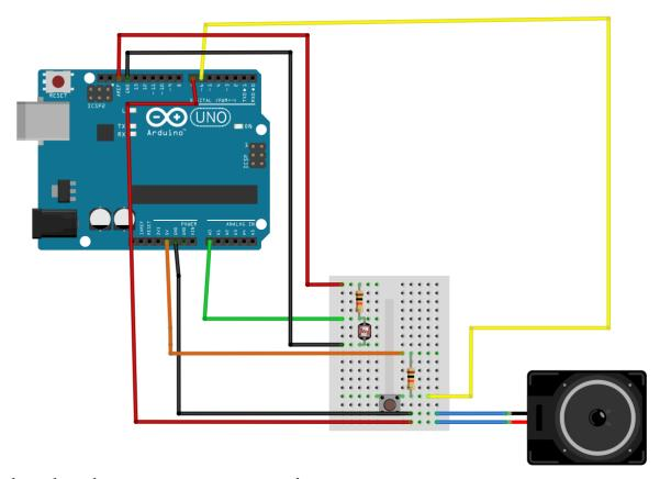
This shows how the components are connected.
