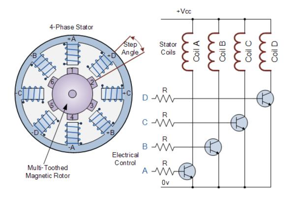
This figure shows how a stepper motor works. The coils are arranged around the outside of the motor, with a permanent magnet rotor in the middle. Each of the coils can be magnetised. If you do this in the right sequence you can make the rotor in the middle "chase" the moving magnetic field and turn.
