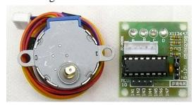
You should have a motor and a board like the ones above. The driver board may look slightly different, but it should have pins labelled IN1, IN2, IN3 and IN4. These correspond to the signals for the four coils you can see above. The board should also have a pair of pins that you can use for power input. One should be marked + and the other – The board also has some LEDs which will confirm when the coils are being driven. The motor plugs into the board.
