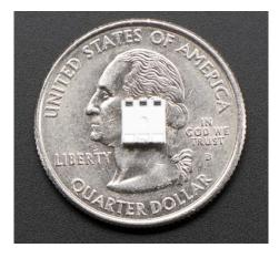
A single NeoPixel device is absolutely tiny, as you can see. They can be used in a daisy chain arrangement, with the output of one linked to the input of the next. A single Arduino pin can be used to control a very large number of lights in this way. Software in the Arduino waggles the data line up and down to signal the amount of red, green and blue the led is to display. When one led has acquired its settings it then passes the signal onto the next one in the chain, and so on.
