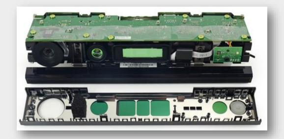
The Kinect V2 builds on the previous device and adds an infra-red camera to the device
